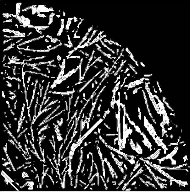
Fig. 4. Simulated transmission electron micrograph of stained structure from a mature spherulite octant. The coordinate system is scaled in lattice units.
